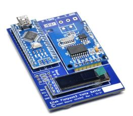
CAN bus data is displayed on the OLED and can be shown on-demand via the serial terminal.
