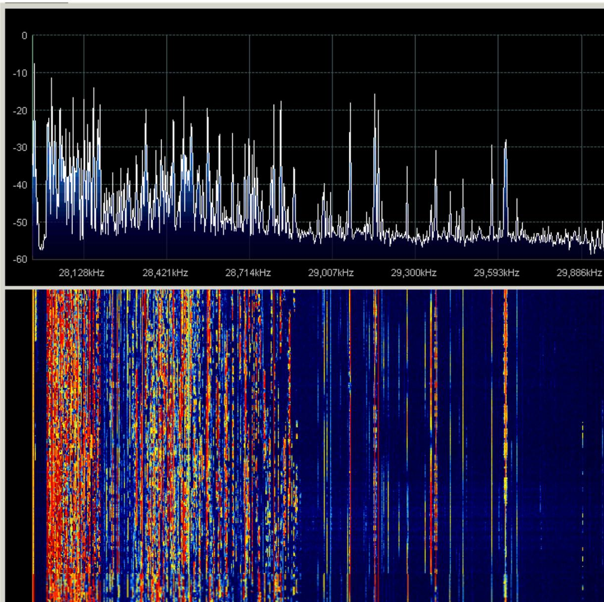
As part of this assessment I've also been testing to see if the limited dynamic range can provide adequate performance on the more crowded bands such as 7MHz. For these tests I have used a passive broadband vertical antenna in conjunction with an up-converter and RTL820 dongle. I used SDR Sharp with various gain settings but no AGC selected. In order to find a worst case scenario with very high level signals I chose frequencies near the 9MHz AM broadcast band.
