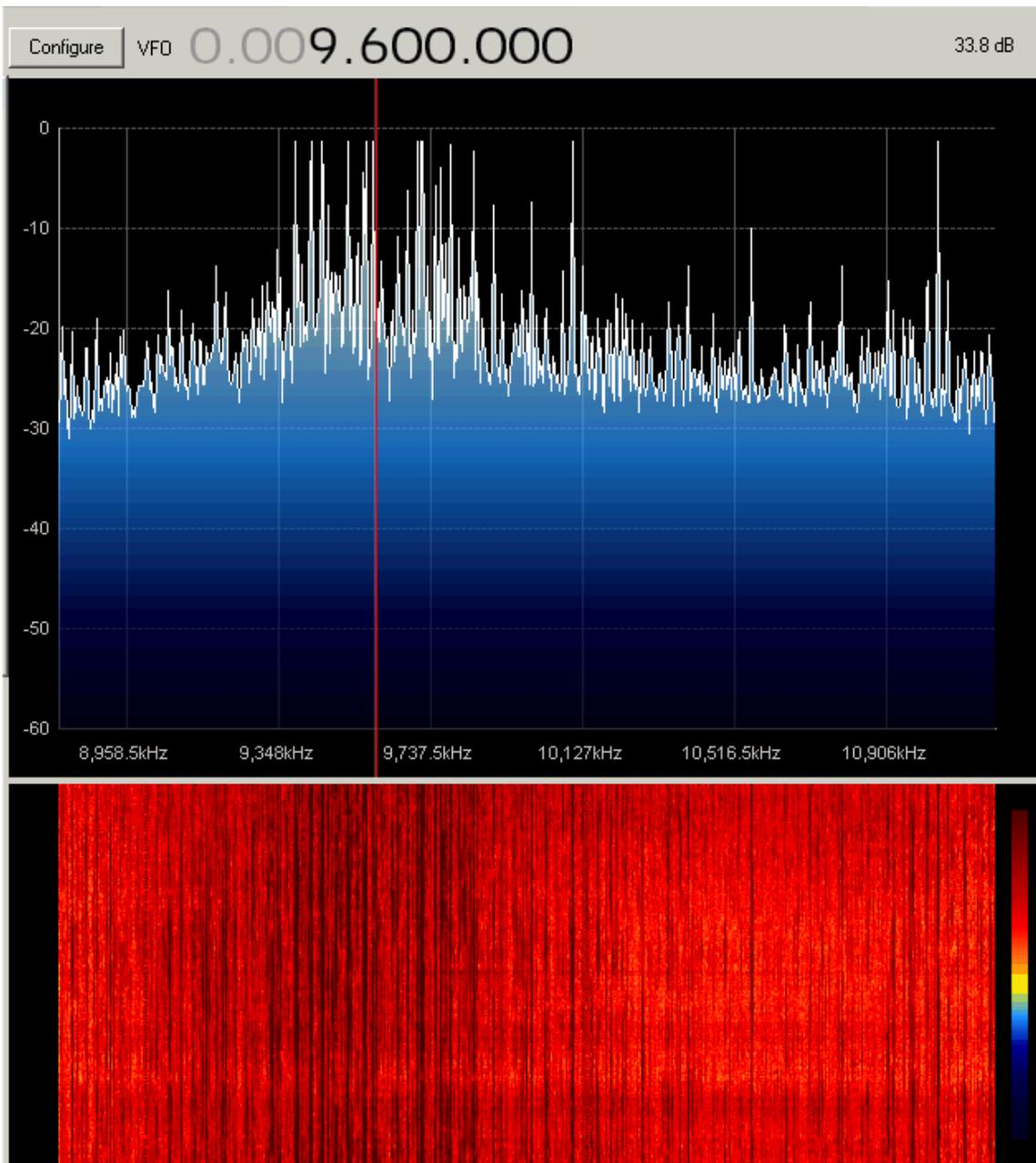
Finally 44dB gain - note the levelling off of maximum signal levels and excessive intermodulation products
