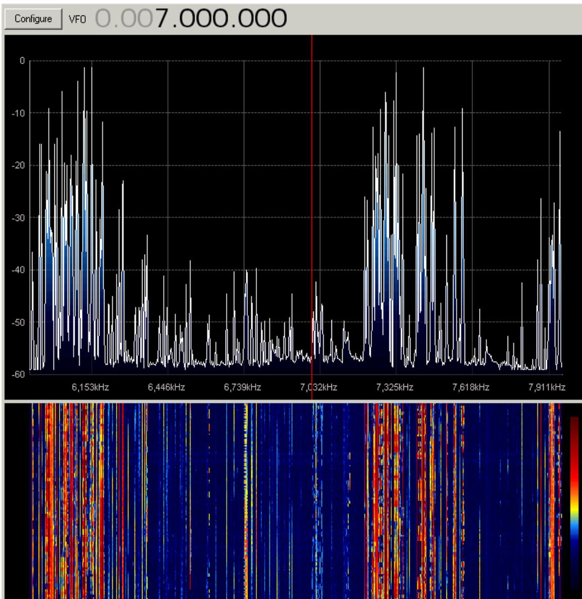
I also performed some two tone IMD measurements on the RTL DVB-T RTL 2832U / Rafael Micro R820T dongle.
