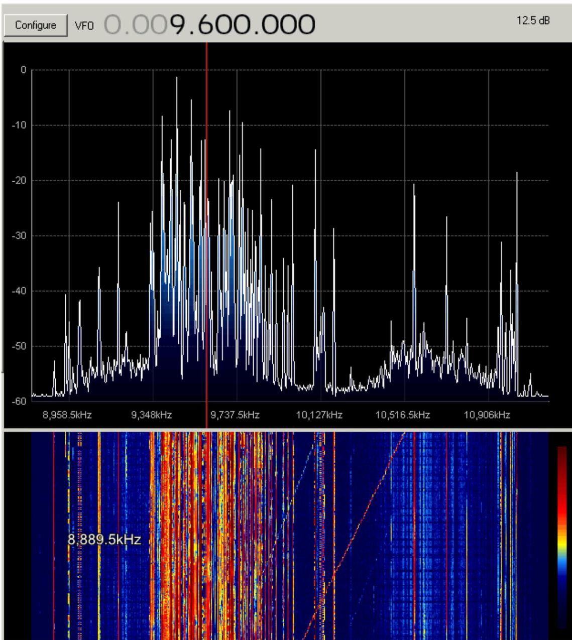
21dB gain - note the rising level of noise floor relative to maximum signals - Start of severe intermodulation and reduction to 40dB dynamic range
