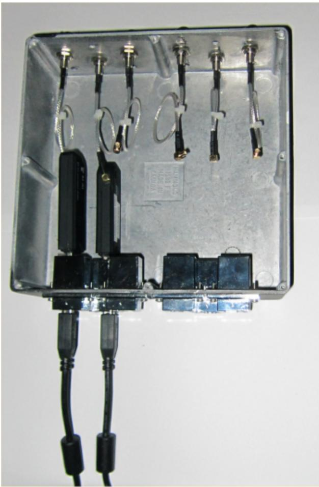
The USB screen needs a good low Z connection to the box metalwork and to the RF connector on the box. I found that if I didn't do this the screening was not as effective. Also any AC potential difference between the antenna coax and PC chassis resulted in current flow across the RTL PCB. This added multiple 50 / 100Hz noise sidebands to the LO.
