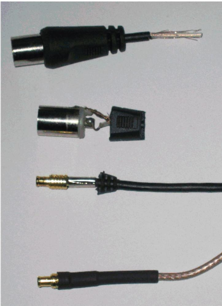
Fortunately it's easy to take apart the crimped connector at the MCX end and fit to some proper PTFE coax. So this is what I've now done rather than wire directly to the board.
