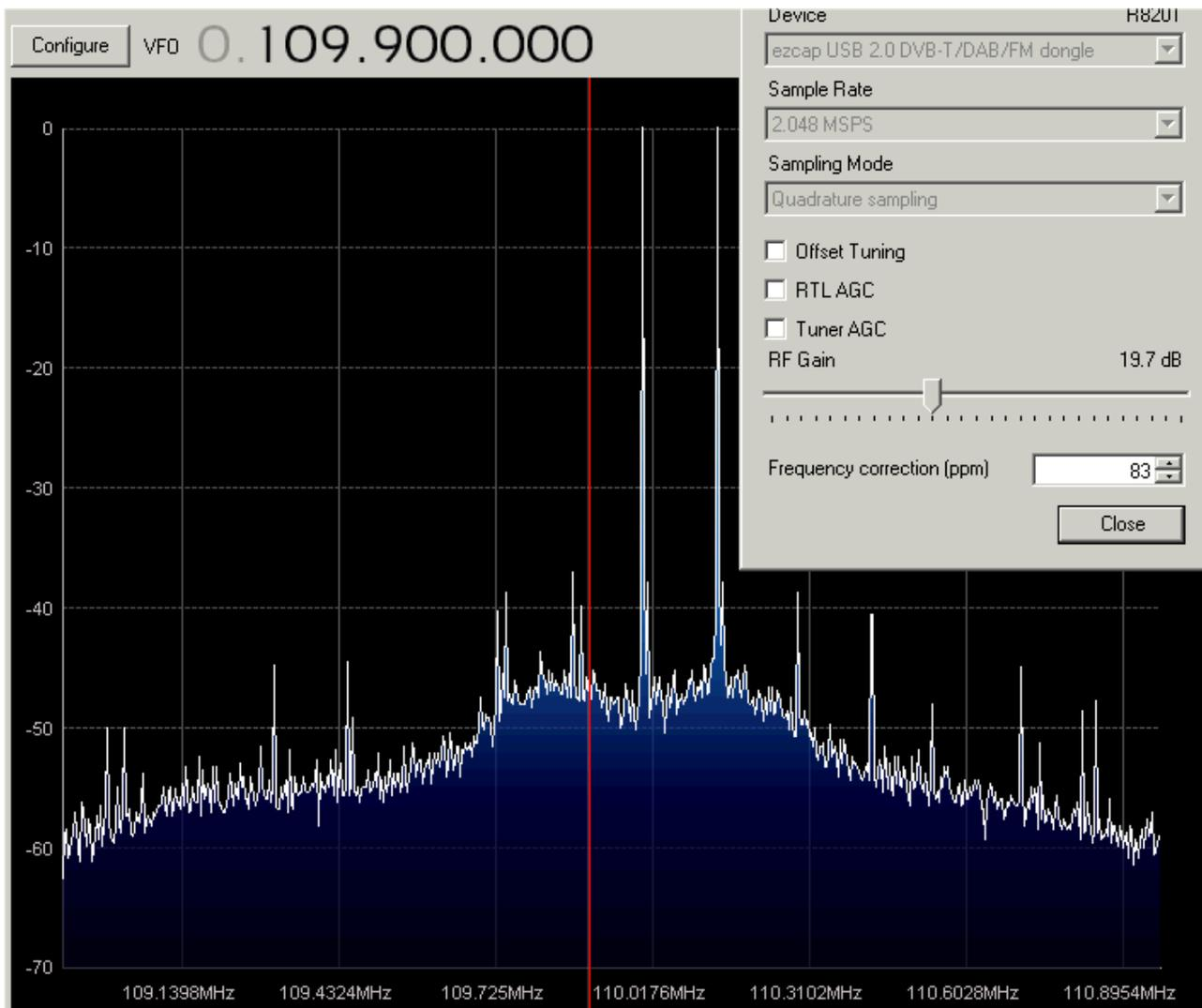
I believe this demonstrates that if the SDR dongle gain is set appropriately, it's perfectly possible to use them for reception of the HF bands with a simple block up-converter.
