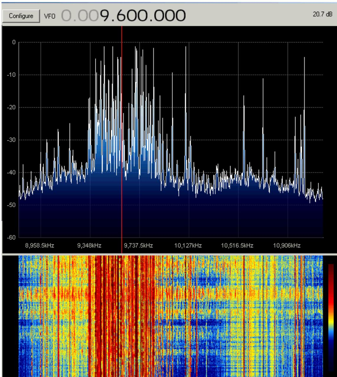
34dB gain - note the very high level of noise floor in relation to maximum signals - very bad intermodulation products and only about 25dB dynamic range
