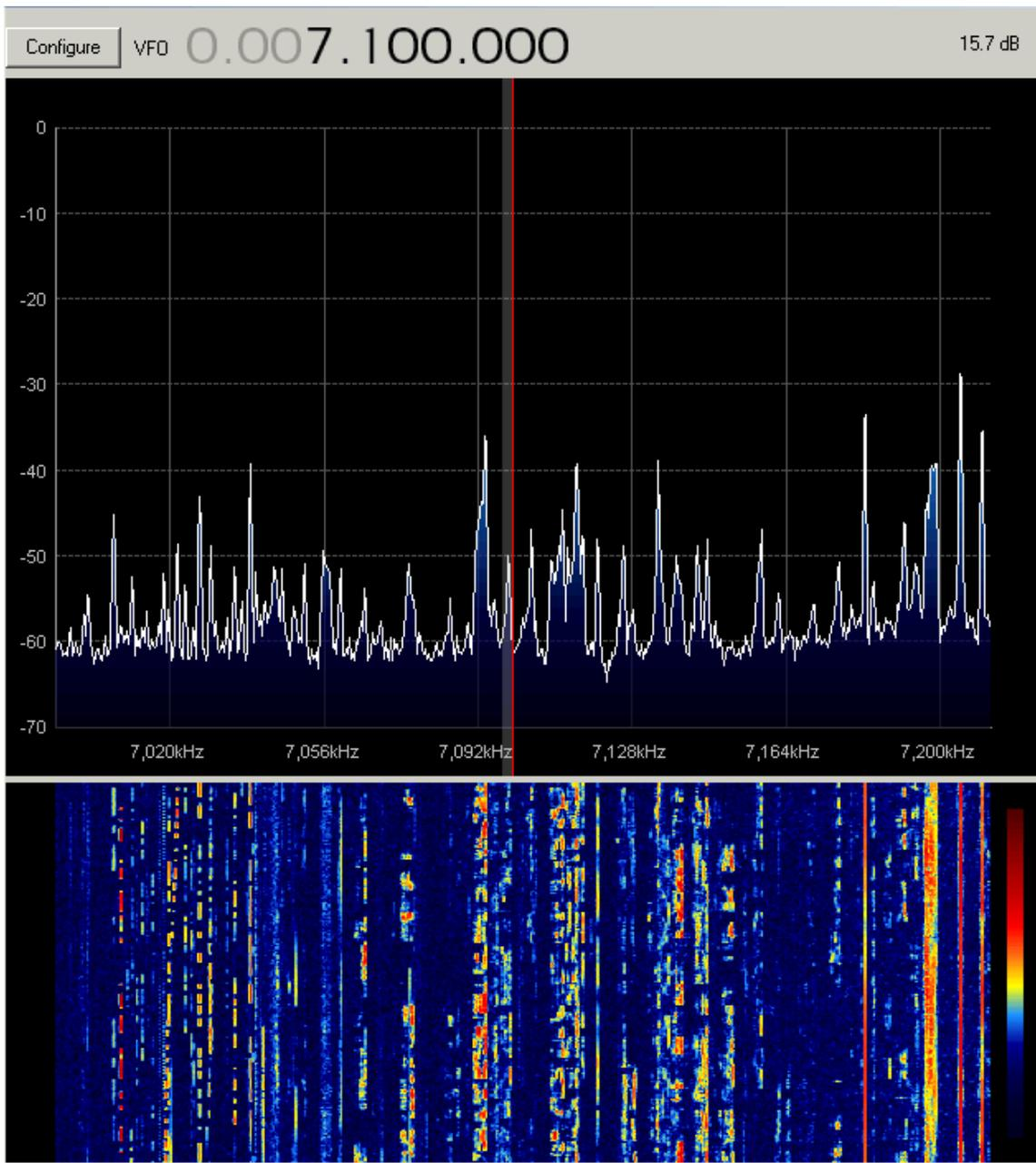
Just to prove that I wasn't cheating with the above screen grab, here's a wider view of the night-time spectrum, with high power broadcast stations either side of the 40m amateur band.
