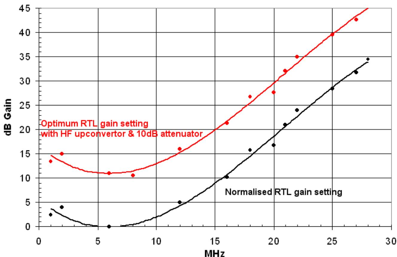
The shape of the general gain / frequency curves tend to remain fairly consistent between day and night. The only real difference is that the overall gain has to be reduced by about 10dB at night to prevent overload at some frequencies between 5 and 15MHz.
