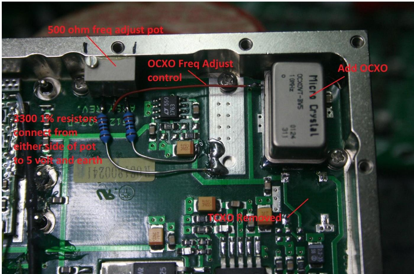
Glue a 500 Ohm 10 turn potentiometer to the side of the case as shown, then connect 3300 Ohm 1% metal film resistors from either side of the potentiometer to both the 5 volt rails and earth. The voltage divider gives a fine tuning range allowing the frequency to be more easily set. From the center winding of the potentiometer connect a wire to the control voltage pin of the OCXO.
