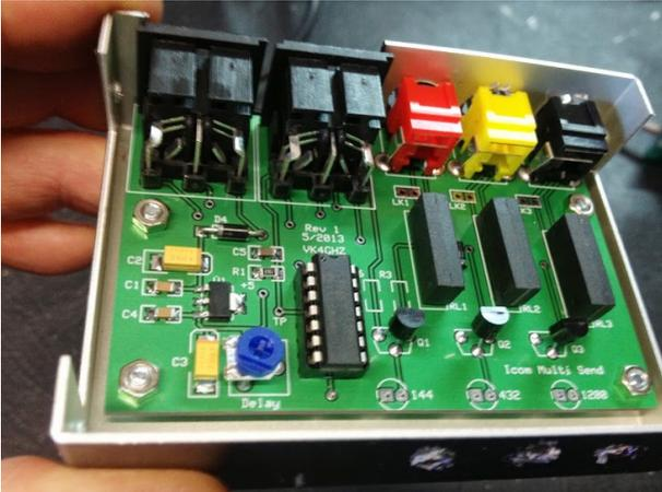
It is recommended that the rear connections be completed first. The instructions indicated drilling separate 17mm holes for the DIN sockets, but I found it easier to cut a square section from the rear panel and file to final size.
