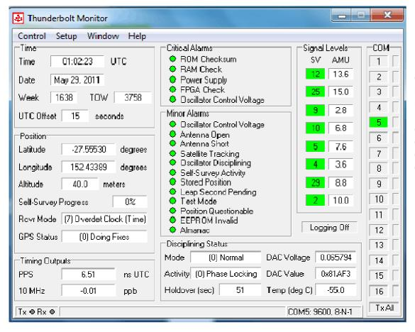
Good signal levels received, and 10MHz output error of 0.01 ppb easily obtained.
